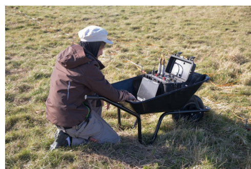
Data Acquisition during the ERT survey: A long cable with 64 electrodes was spread out several times to measure the apparent electrical conductivity of sediments along a transect of 145 m.
