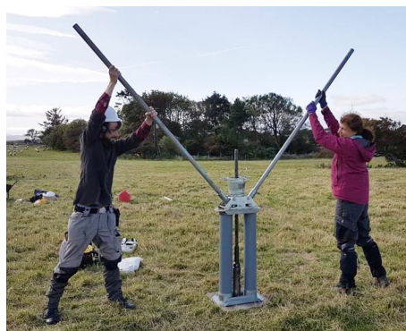
Core extraction: Two persons and long levers are needed to retrieve the cores from depths of up to 3.5 metres.
