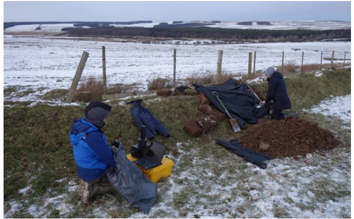
Soil samples collected under a dark cover from a field boundary near Gallows Hill farm are immediately analysed using a portable OSL reader (photograph by Soetkin Vervust).
