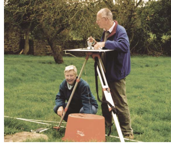
Plane table surveying at Low Harperley
