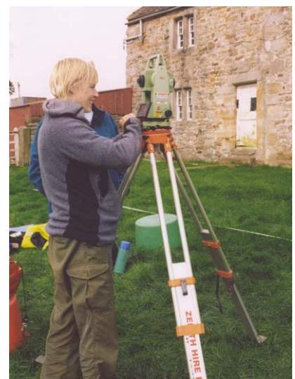
Demonstration of the use of a total station theodolite, Low Harpeley, by AASDN Fieldwork Co-ordinator, Penny Middleton
