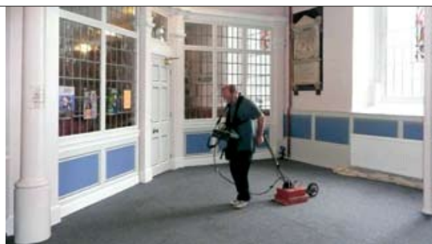
Brian Donnelly of Northumbrian Surveys carrying out his GPR survey in the visitor centre of St Hilda's Church
